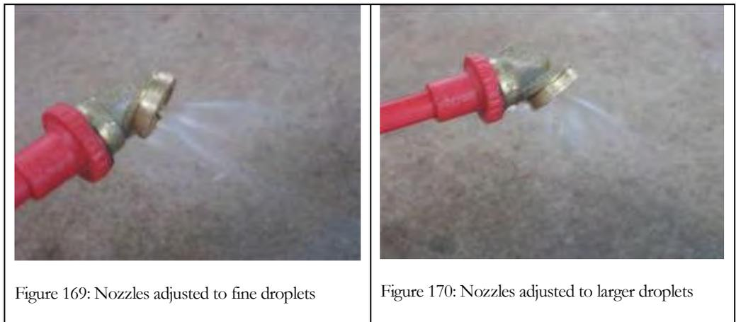
Figure 169 shows the nozzles adjusted for fungicide application, the spray is as fine as possible with this type of knapsack sprayer. Figure 170 shows the nozzles adjusted for herbicides and certain insecticides.
