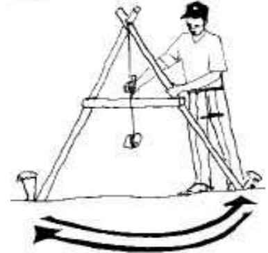
Figure 75: Calibrating the A-frame
