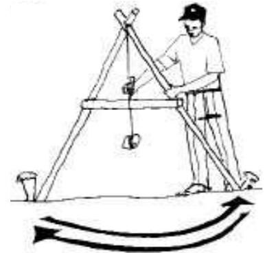
Figure 75: Calibrating the A-frame
