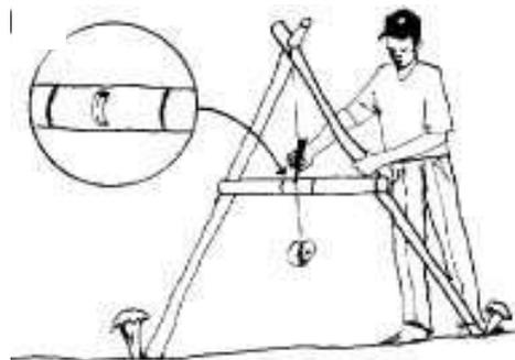
Figure 76: Using an A-frame
