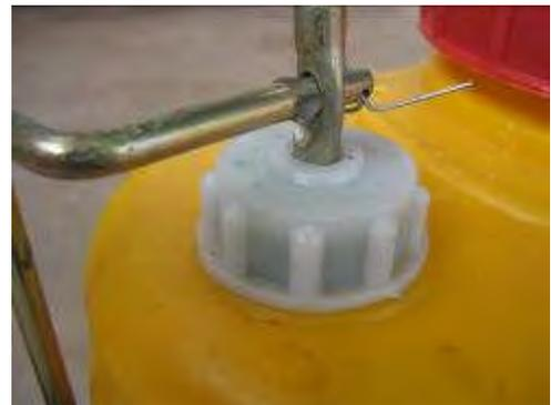
Figure 166: Old knapsack sprayer with some leaking connections
